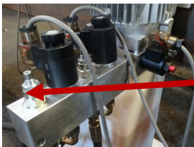
throttle valve controlling refilling of the primary platform
